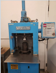
SUPERPAVE GYRATORY COMPACTOR
